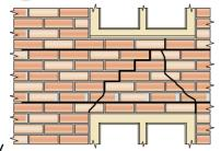
Parallel lengths of HeliBar rod are bonded into the specified slots, cut above the existing lintel, and finished with matching pointing.
